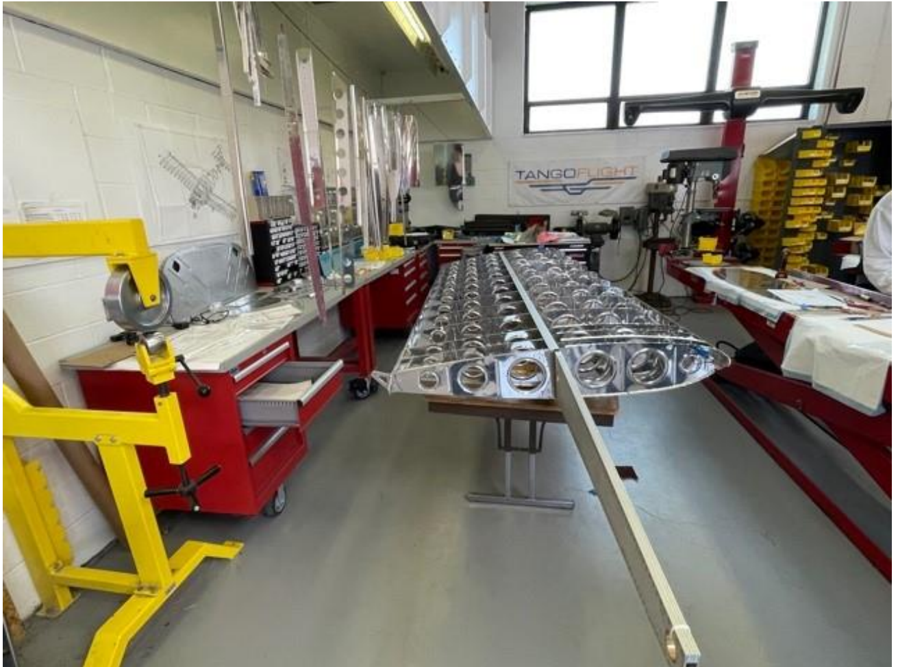
Figure 3 - Wing frame complete
