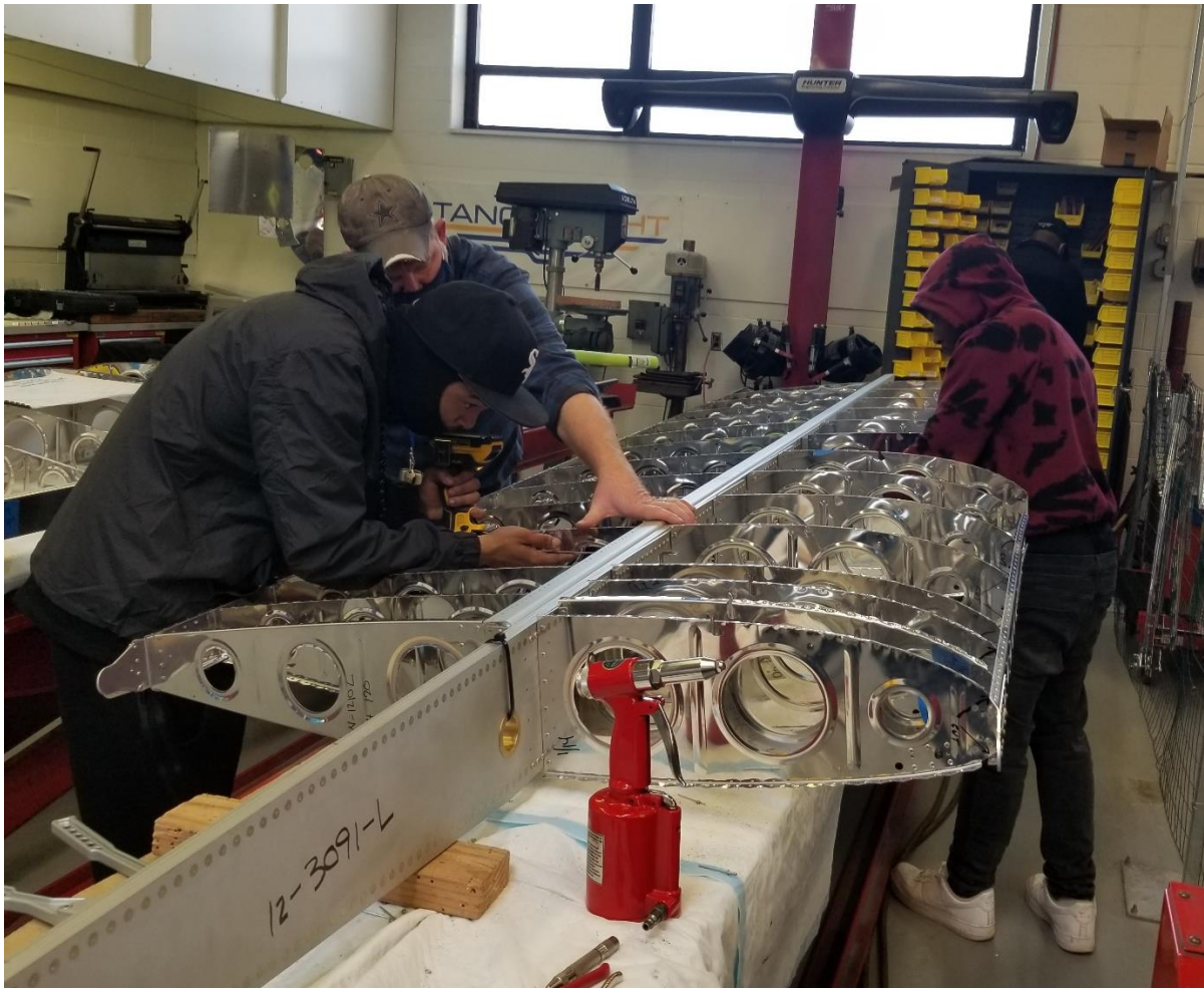
Figure 10 - Students and mentors assembling wing
