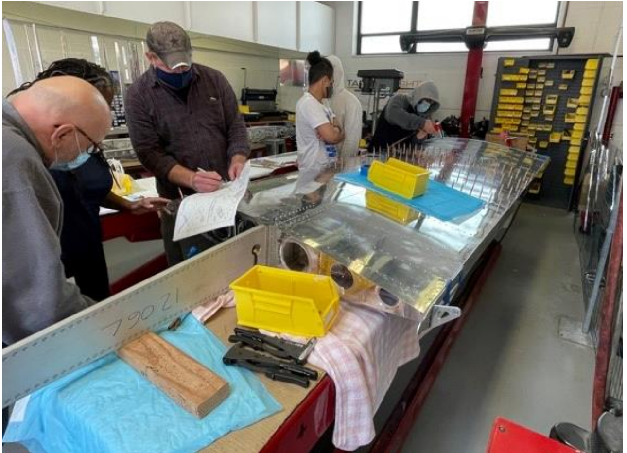
Figure 5 - mentors and students checking plans and riveting wing shell
