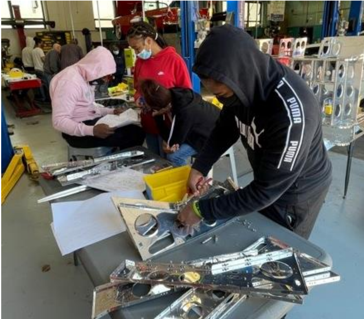
Figure 2 - Students assembling wing frame
