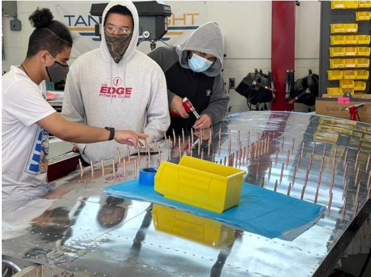
Figure 1 - Students riveting wing
