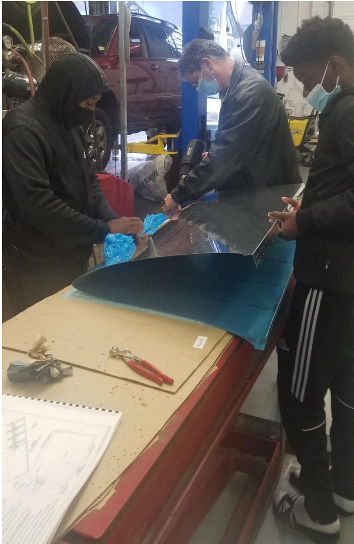
Figure 7 - Students bending sheet metal for tail wing
