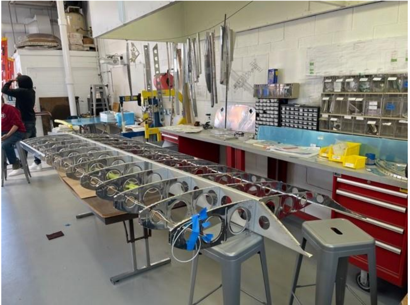
Figure 4 - Wing frame with wiring
